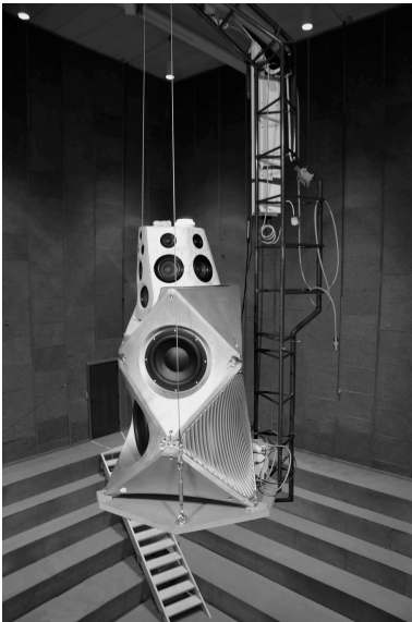
Figure 9.1: The first Beolab 90 prototype undergoing acoustical measurements in The Cube.
